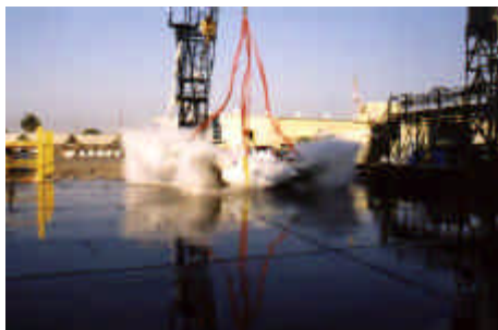
Figure 2 Linear Tank Catastrophically Failed
